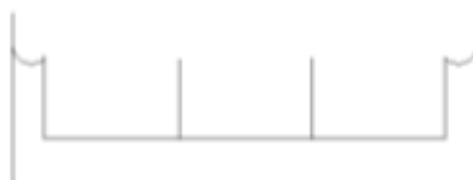
c) 敞口隔舱式内浮顶
